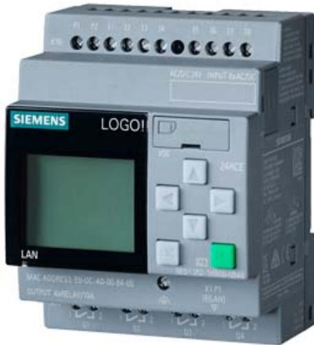
LOGO! 24RCE, MOD. LOG., DISPLAY AL/E/S: 24V AC/24V DC/RELE, 8 ED/4 SD, MEM. 400 BLOQUES AMPLIABLE MODULARMENTE, ETHERNET WEB-SERVER INTEGR., DATALOG, TARJETA MICRO SD ESTANDAR PARA LOGO! SOFT COMFORT >= V8 PROYECTOS ANTIGUOS EJECUTABLES
